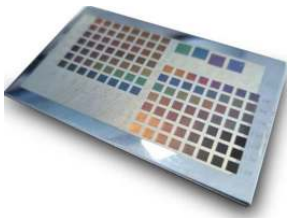
Color Marking on Stainless Steel
